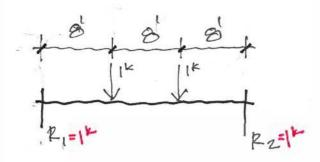
5hear for wood  $f_V = \frac{3}{2} \frac{1}{4} = \frac{3}{2} \times \frac{1 \times 1000 \text{ LB/K}}{1.5 \text{ IN} \times 11.25 \text{ IN}}$ = 89 PSI < 180 Or/
